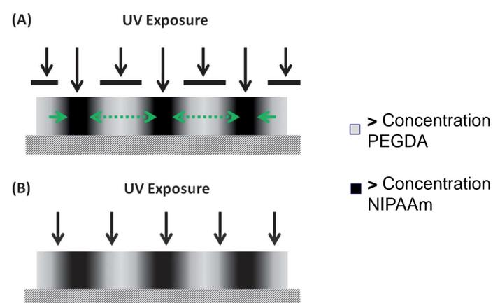
Figure 3: Fabrication steps of hydrogel coatings with switchable surface topologies. (A) Maskwise exposure. Green arrows indicate NIPAAm diffusion to the exposed area. (B) All remaining acrylates are polymerized during flood exposure. [2]
