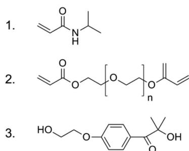
Figure 2: The PNIPAAm hydrogel is made from 1. Monomer N-isopropylacrylamide (NIPAAm), 2. Crosslinker Polyethylene glycol diacrylate (PEGDA), 3. Photo initiator Irgacure 2959. [1]
