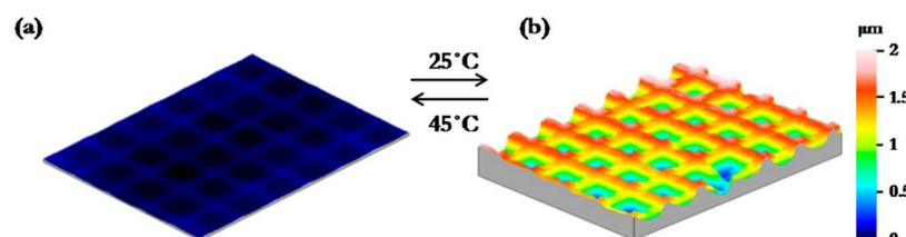
Figure 4: Interference microscopy 3D images showing surface topographies of a poly(N-isopropylacrylamide) coating cycled between warm(a) and cold(b) water. [1]
