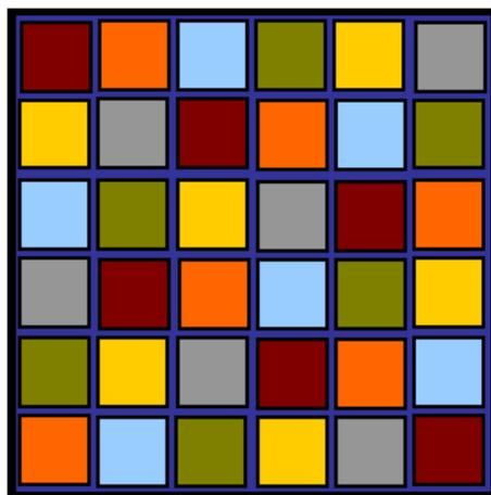
Figure 1: Latin square coating layout, with the 6 colours representing 6 coatings
