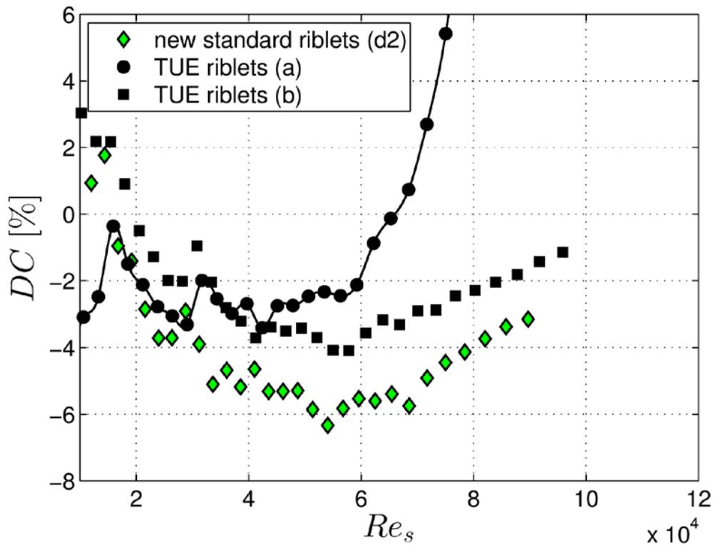
Figure 2 Drag change for the fluoropolymer riblet coatings.
