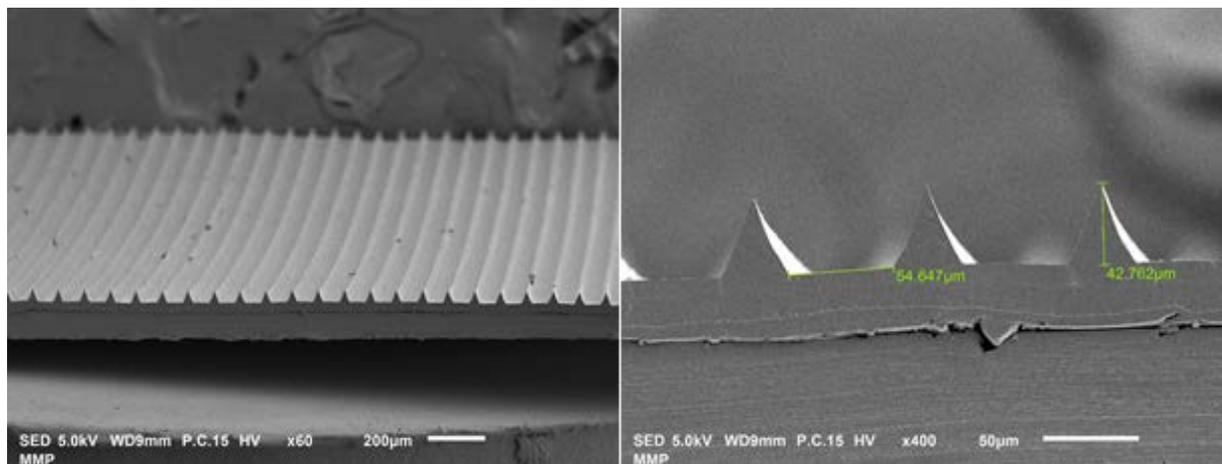
Figure 1 SEM images of the cross-linked fluoropolymer riblet coatings developed by Technical University Eindhoven in collaboration with Fraunhofer IFAM. Source: Technical University Eindhoven.
