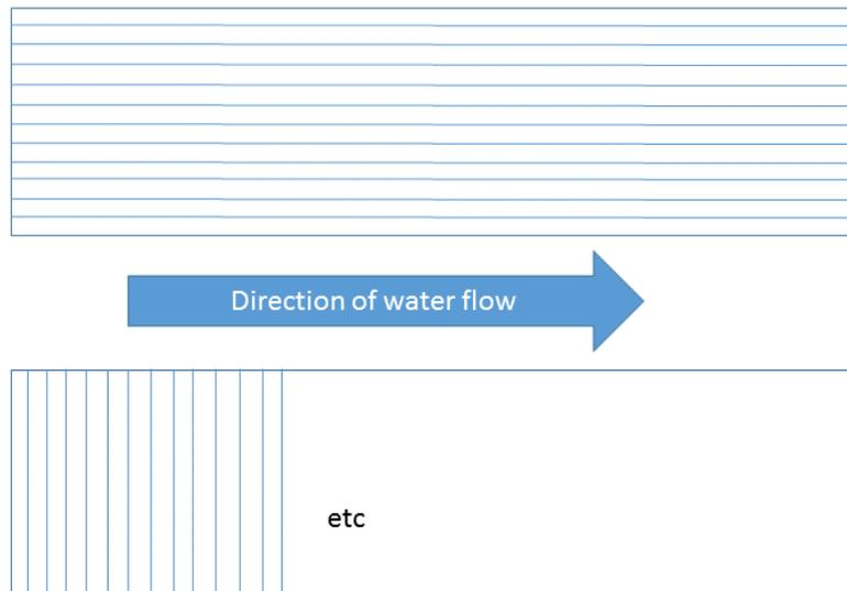
**Figure 4: Illustration of the two different riblet orientations prepared on the microscope slides. The arrow indicates the direction of the water flow in the test facility for diatom removal.**
