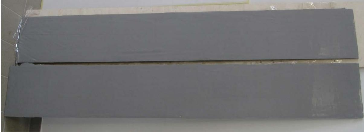
Figure 3: Photo of the two Plexiglas plates equipped with smooth **solvent-free IS 1100SR** for water tunnel testing.
