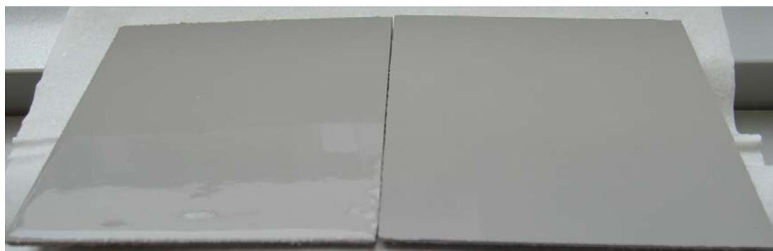
**Figure 5: Photo of two PVC plates coated with **solvent-free IS 1100SR** with a shiny smooth (left) and an opaque riblet-textured surface (right).**
