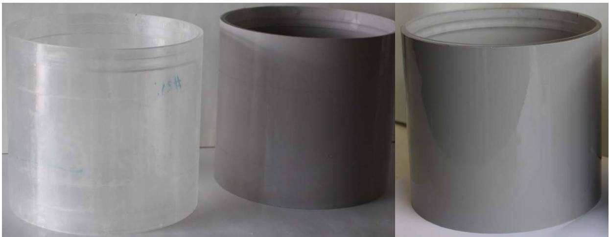
**Figure 2: Photos of the three types of coated cylinders for Taylor-Couette testing in WP1.1.3:** Riblet-textured dual-cure paint from Fraunhofer IFAM (left), riblet-textured solvent-free IS 1100SR provided by AkzoNobel (centre), and smooth solvent-free IS 1100SR (right). For each type, two replicates were manufactured and provided to TU Delft.
