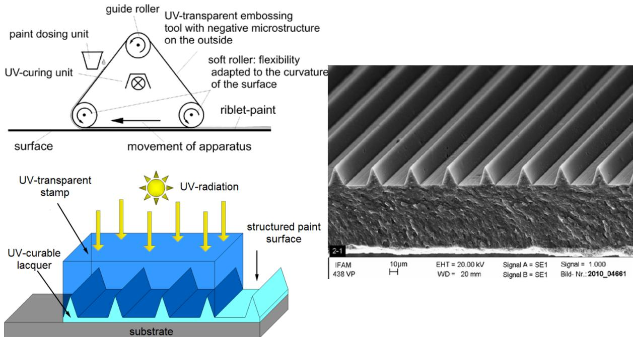
**Figure 1: Schematic of the continuous embossing-curing technology developed by Fraunhofer IFAM:** Principle of the automated application device (top left), schematic of simultaneous embossing and curing mechanism (bottom left); REM image of resulting riblet-textured coating (right).
