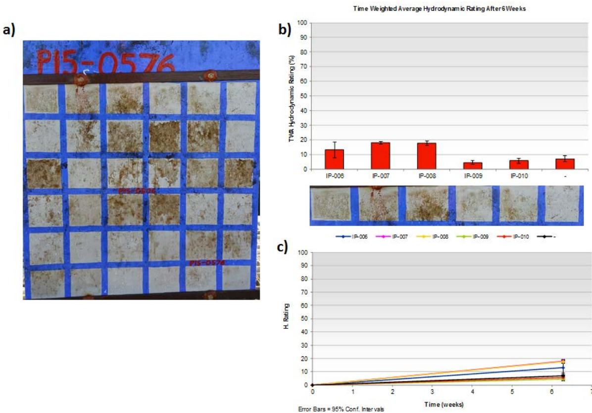
**Figure 2:** 6 x 6 Latin square board after 6 weeks immersion in Hartlepool, UK (a), time-weighted average hydrodynamic fouling rating for each coating at 6 weeks (b); H-rating as a function of time.
