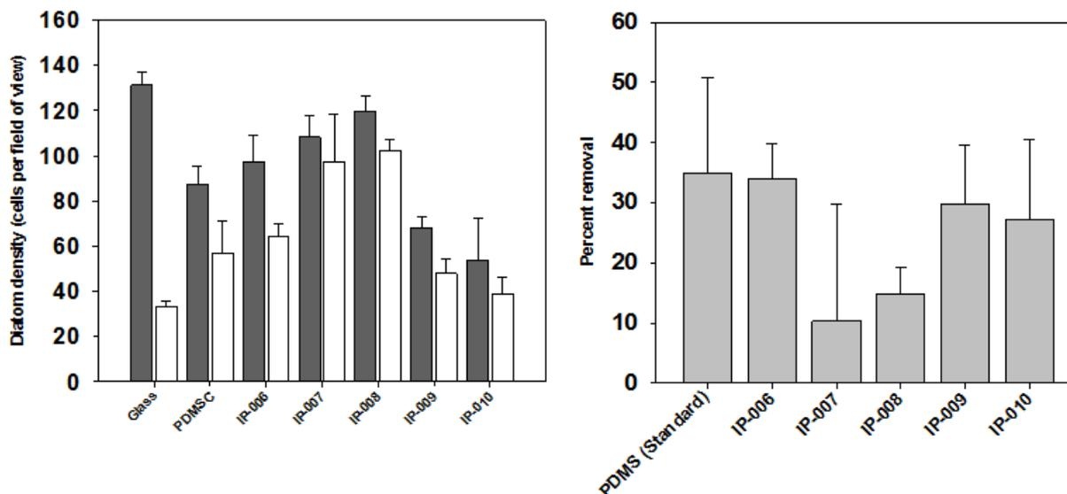
**Figure 6:** Density of diatom settlement before and after application of hydrodynamic shear (a), percentage of diatoms removed by application of hydrodynamic shear (b).
