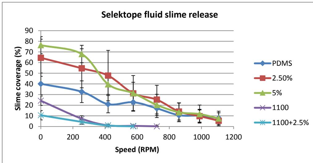
**Figure 4.** Slime coverage as a function of shear water speed (water speed represented by the pump impeller speed in RPM).
