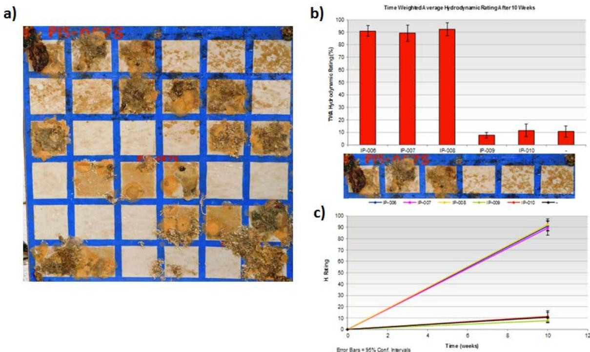
**Figure 1:** 6 x 6 Latin square board after 10 weeks immersion in Singapore (a); time-weighted average hydrodynamic fouling rating for each coating at 10 weeks (b); hydrodynamic (H) rating as a function of time (c).
