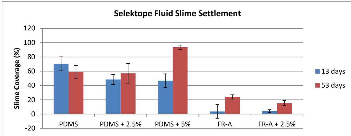
**Figure 3:** Slime coverage of glass microscope slides coated with IP006-010 after 13 and 53 days in Dove marine laboratory 'slime farm'.
