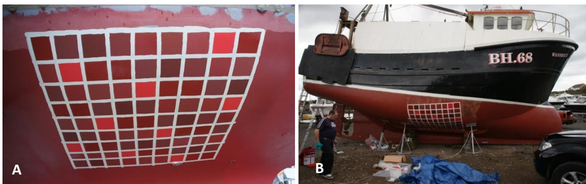
Figure 1. Experimental design used in the study. A – Latin square board with the nine coatings. B – Test area located on the starboard hull of a vessel.
